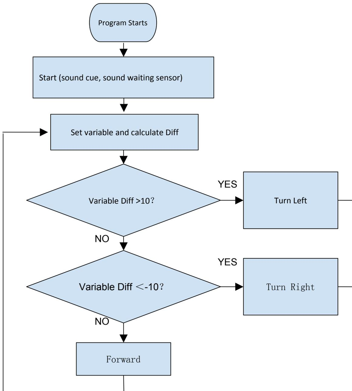
Connect the computer with Bluetooth to start the program and then the robot will turn with the light of flashlight. Put the flashlight right ahead of Ranger and the robot will advance slowly.
